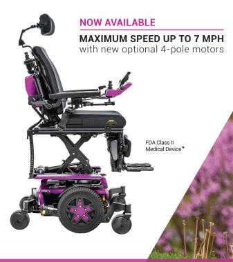
Upgraded SRS (Smooth Ride Suspension) provides a smooth, comfortable ride and advanced stability. Optional iLevel® is available at 4.5 mph with up to 12" of power adjustable seat height. Standard features include front and rear LED fender lights, a USB charger, and drive wheel color accents. TRU Balance® 4 Power Positioning with anterior tilt and memory seating.
