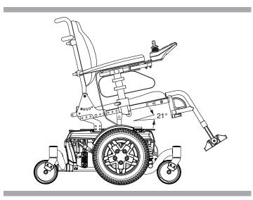
Figure 10. Seat Angle (Dump) Adjustment
