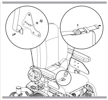
Figure 16. Positioning Belt Installation and Adjustment
