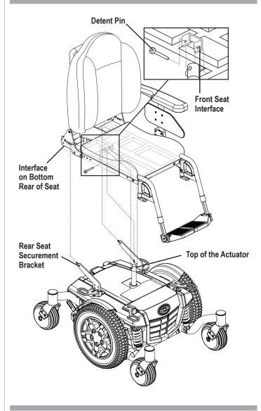
Figure 4. Mounting System and Contour Seat
