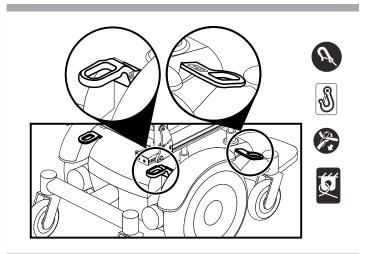
Figure 6. Transit System Securement Brackets
