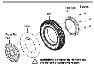
Figure 21. Q4 Drive Wheel Disassembled
