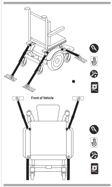
Figure 7. Unoccupied Transit System Securement Points
