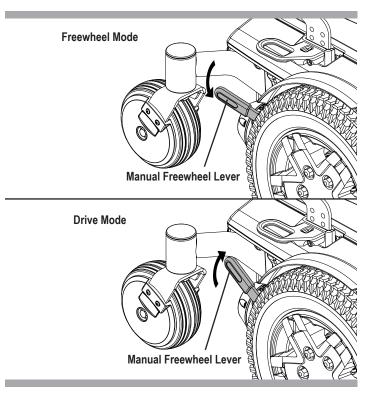
Figure 2. Manual Freewheel Lever Operation
