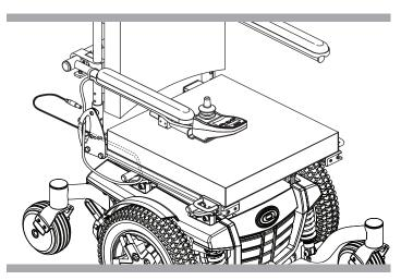
Figure 5. Controller Harness Routing on a Synergy Seat
