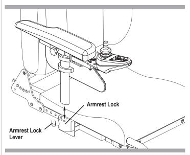
Figure 13. Armrest Removal, Installation, and Top Height Adjustment
