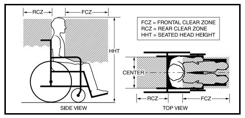
Figure 5. Recommended Clear Zones for Wheelchair-seated Occupants
