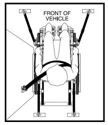
Figure 1. Securing the Wheelchair
