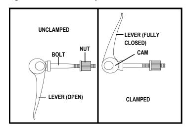
Figure 21. Quick Release Fastener Operation
