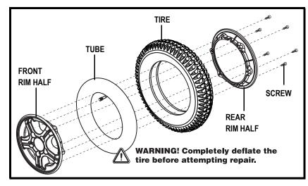
Figure 25. Quantum 600 Series Drive Wheel
