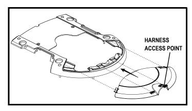
Figure 12. Rear Shroud Assembly
