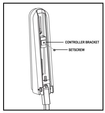
Figure 19. Underside of Armrest
