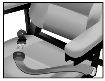
Figure 23. Positioning Belt Adjustment
