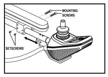
Figure 18. Controller Position Mounting Bracket
