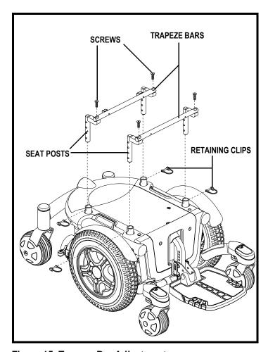
Figure 15. Trapeze Bar Adjustment
