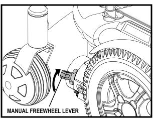
Figure 8A. Drive Mode (Drive Engaged)
