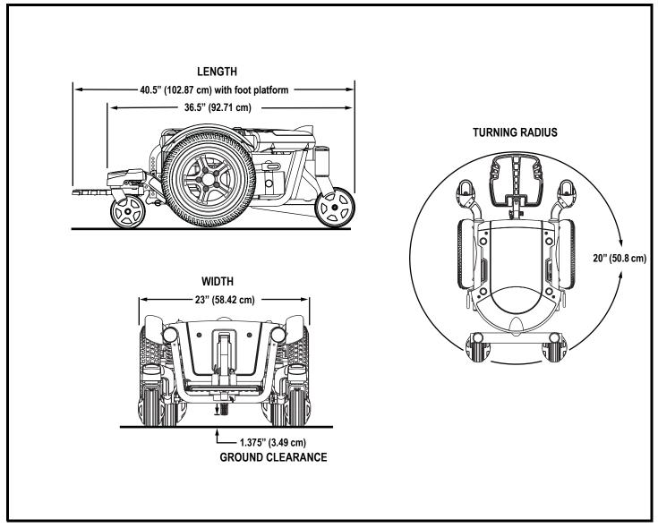
Figure 28. Quantum 600 Series Dimensions and Ground Clearance
