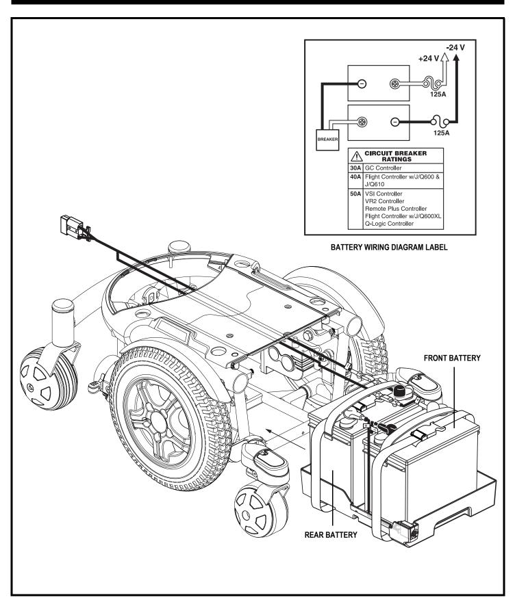
Figure 27. Battery Installation
