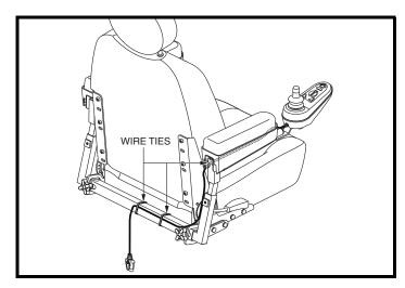
Figure 13. Controller Harness Routing on a Contour Seat
