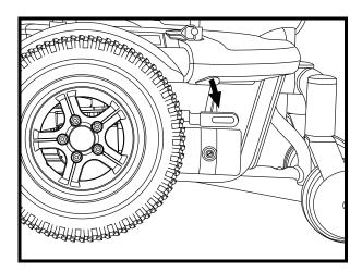
Figure 9B. Freewheel Mode (Drive Disengaged)
