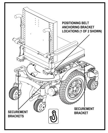
Figure 14. Transit Securement System Brackets
