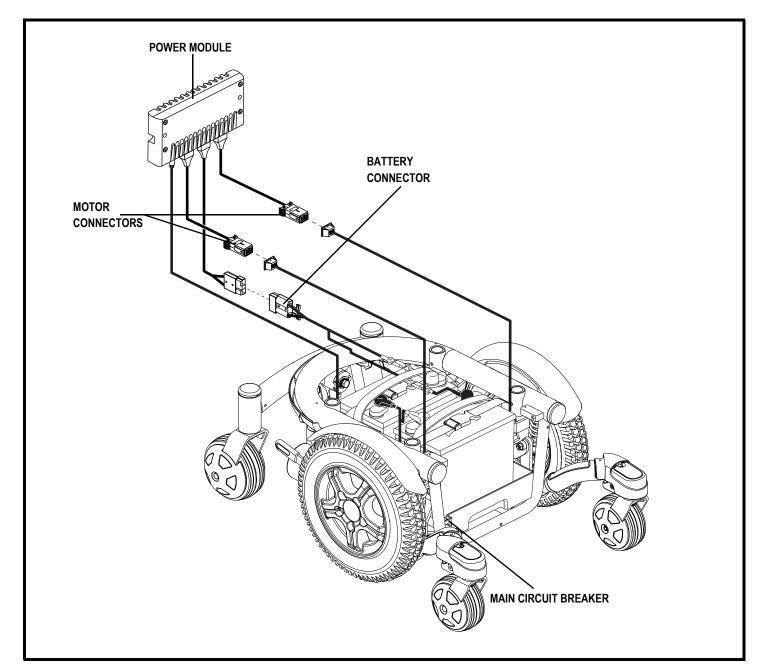
**Figure 7. Electrical Components**
