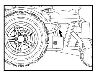
Figure 9A. Drive Mode (Drive Engaged)
