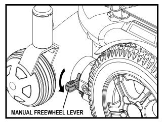
Figure 8B. Freewheel Mode (Drive Disengaged)
