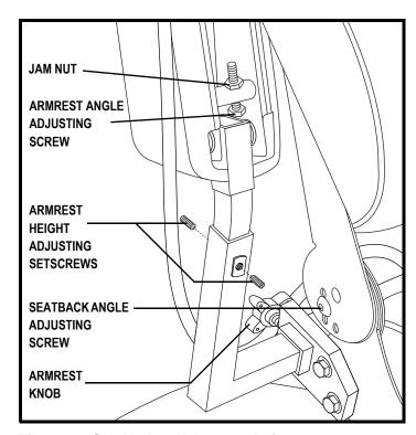
Figure 17. Seatback and Armrest Adjustment
