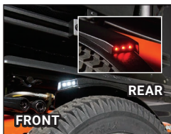
Front and Rear LED Fender Lights
