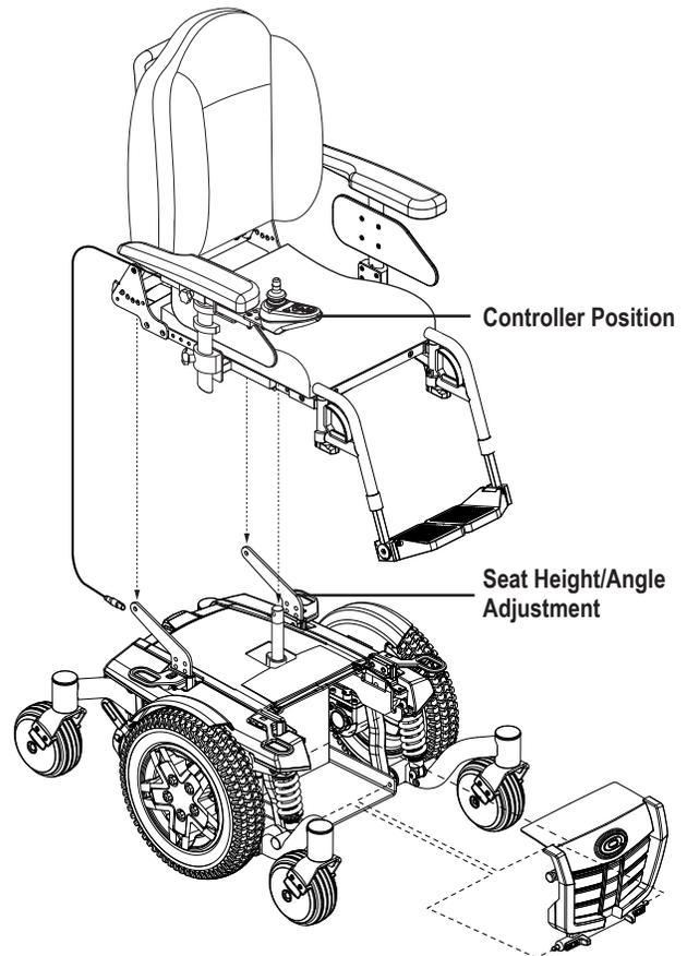
Figure 3. Q4 Assembly View
