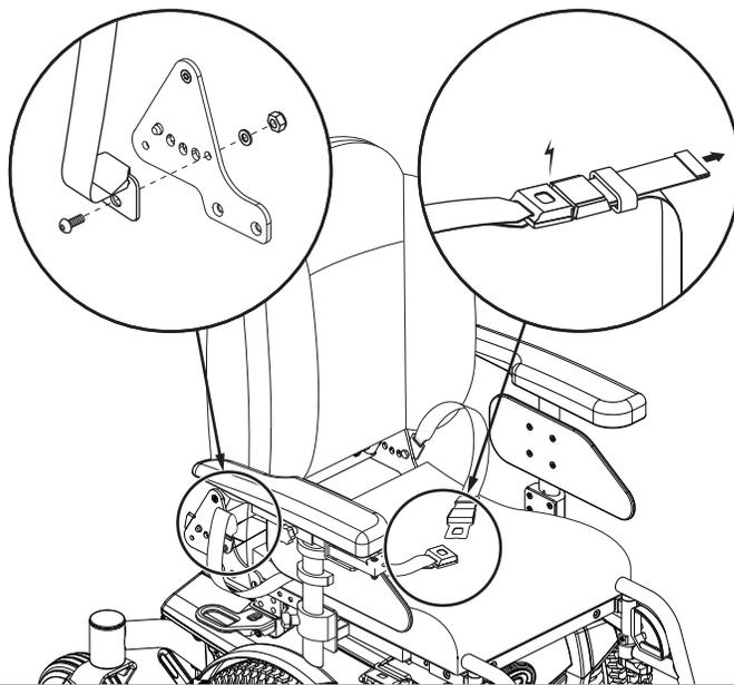
Figure 16. Positioning Belt Installation and Adjustment
