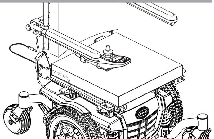
Figure 5. Controller Harness Routing on a Synergy Seat
