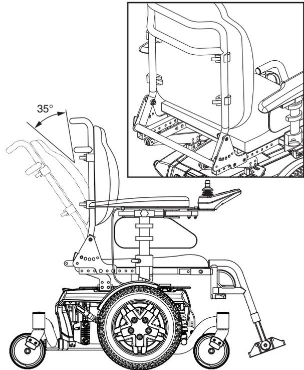
**Figure 8. Manual Recline Seatback Adjustment**
