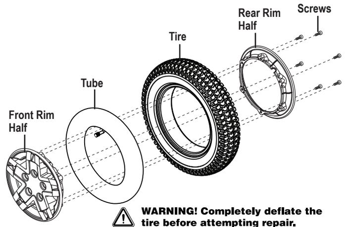
Figure 21. Q4 Drive Wheel Disassembled
