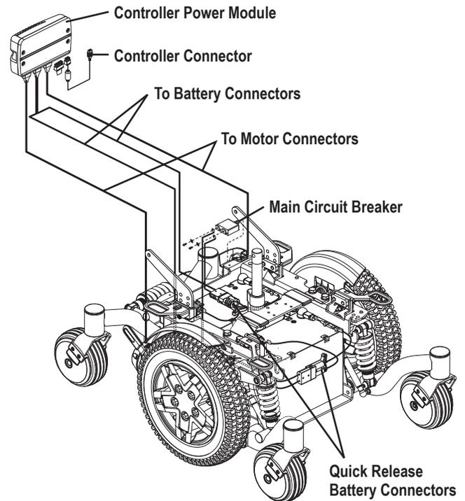
**Figure 1. Q4 Electrical Components**
