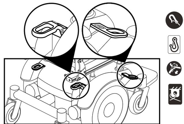
Figure 6. Transit System Securement Brackets
