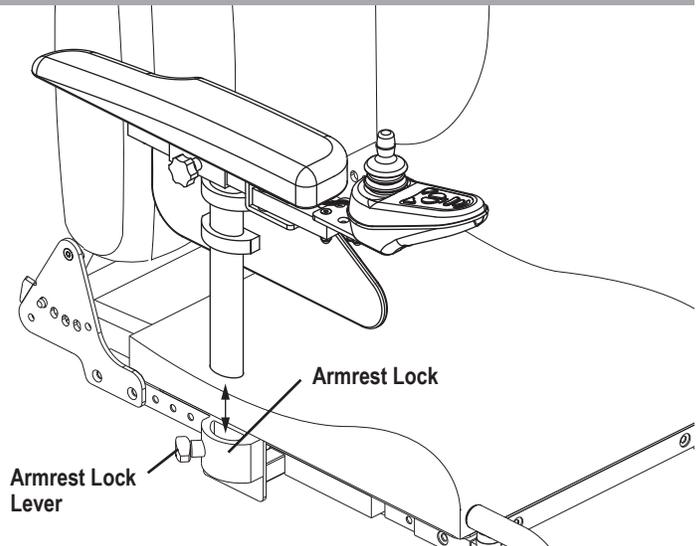
**Figure 13. Armrest Removal, Installation, and Top Height Adjustment**
