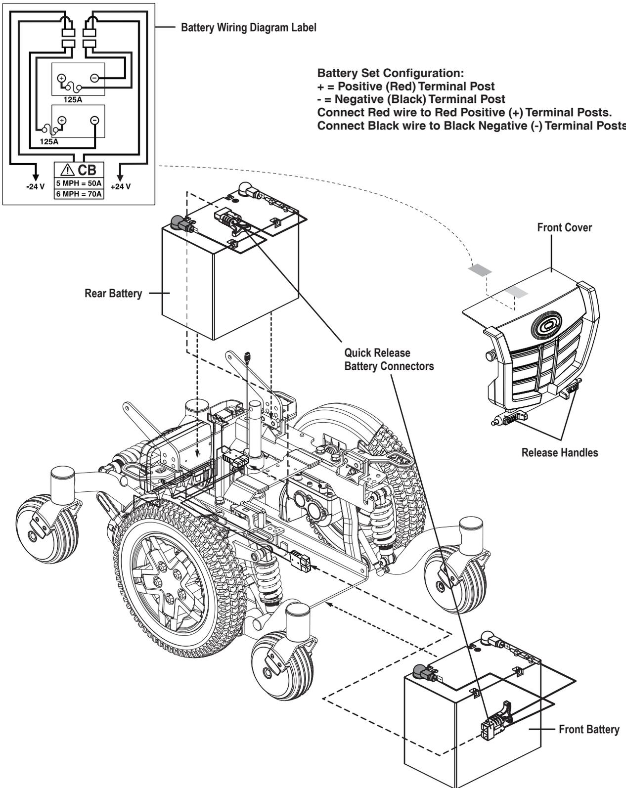
Figure 22. Battery Installation
